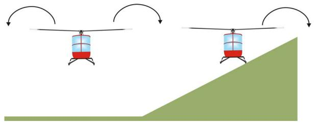
In general dynamic roll-over occurs when the pilot is too harsh and quick on the controls, not noticing that one skid is either stuck on the ground or the pilot has over controlled and caused the helicopter to commences a roll about the skid.
