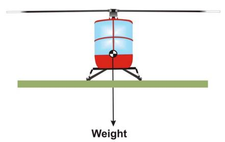
If we were to come along with a bottle jack (the type used to jack up a car when you have a flat tyre) and place it under the skid, you could lift the helicopter up off the ground. One skid would raise, the other would act as a pivot point about which the helicopter would be rotating.
