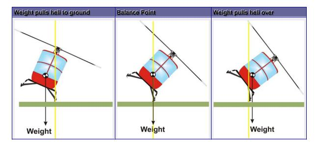
In an R22 the helicopter can reach a critical angle of 42° before it reaches the point where it will roll over. What has been described is static rollover where the helicopter is not under power.
