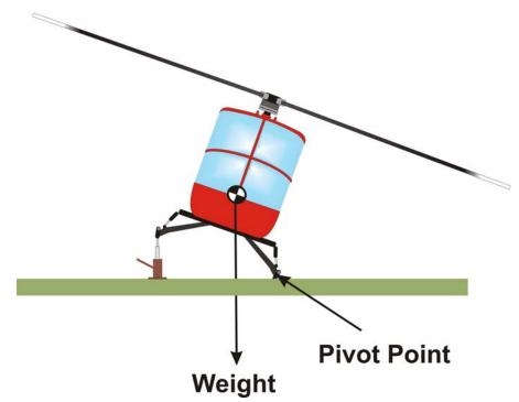
The interesting thing here is, the helicopter will not roll over onto its side until the centre of gravity of the helicopter passes a line running vertically upwards from the pivot point.
